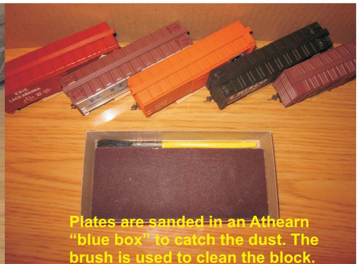
Plates are sanded in an Athearn "blue box" to catch the dust. The brush is used to clean the block.
